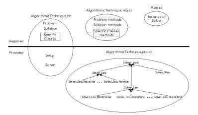
Fig. 1. Architecture of a MALLBA skeleton
