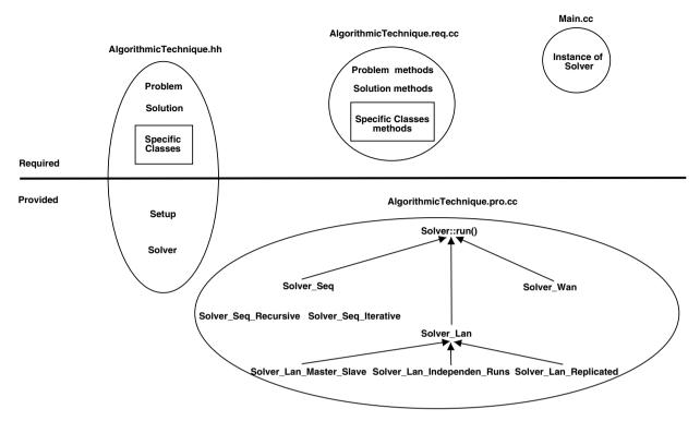
(a) Architecture of a MALLBA skeleton. The horizontal line stands for the separation between the C++ classes the user must fulfill (upper part) and the classes that the skeleton already includes in a fully operational form (lower part).
