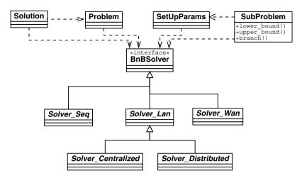
Fig. 3. UML diagram of the Branch-and-Bound skeleton.
