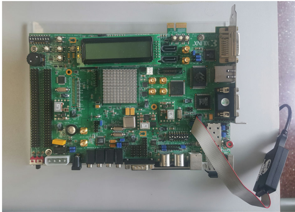
Fig. 5 Picture of the Virtex-5 XC5VLX110T board used for the implementation of the C-Mantec algorithm
