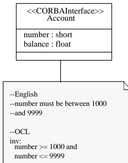
Figure 6. A Fragment of a Semantically Enhanced CORBA Specification
