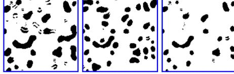
**Fig. 5.** Comparison of two accessibility maps obtained with  $T_1$  (first and center images) and the resulting overlap (right image) - the amount of overlap is 50.07%.
