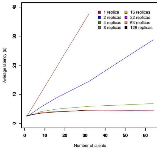
Fig. 4. Average latency response of modal analysis in FogPi with different numbers of replicas
