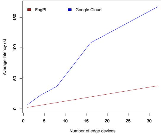
Fig. 3. Average latency response of modal analysis by multiple edge devices in FogPi and Google Cloud
