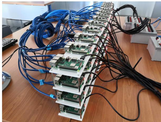
Fig. 2. FogPi: A Portable Fog Infrastructure through a Raspberry Pi cluster
