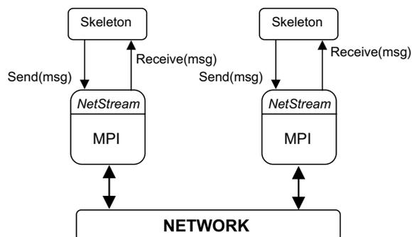
Fig. 2. NetStream communication layer on top of MPI.
