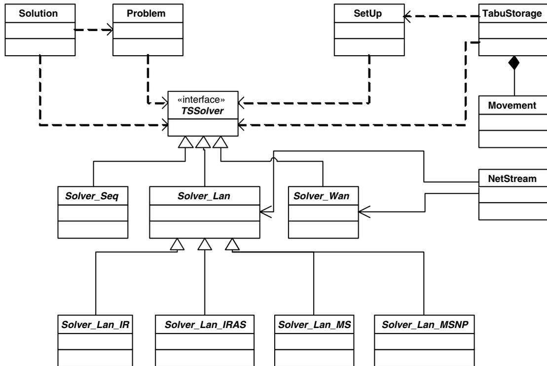
Fig. 4. UML diagram of the Tabu Search skeleton.
