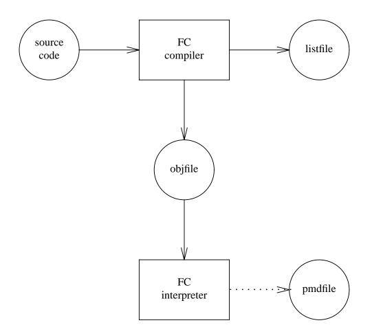
Figure 3.1: Files and Pascal-FC System Components
