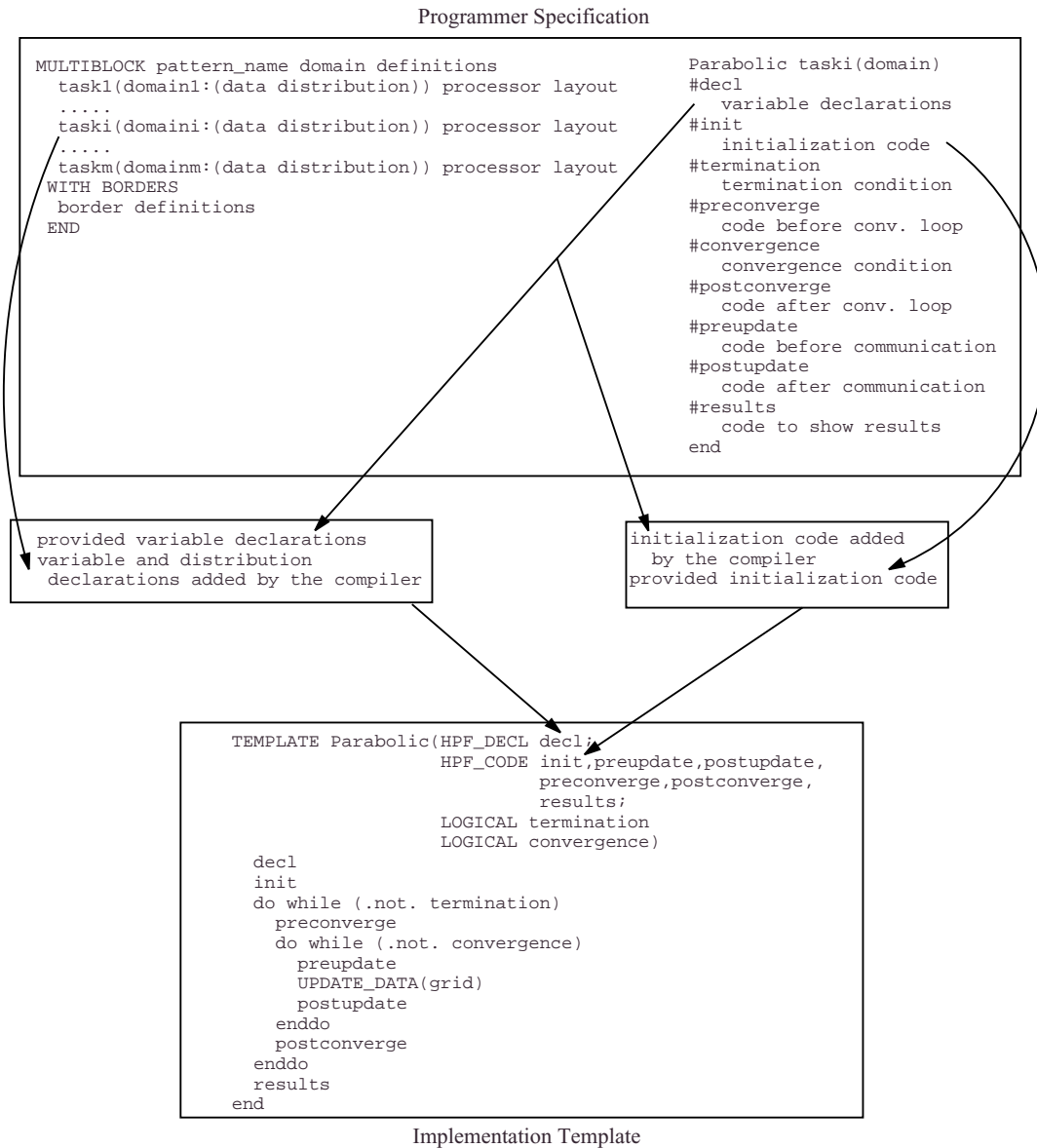
Fig. 4. The Parabolic template and its instantiation from DIP specification
