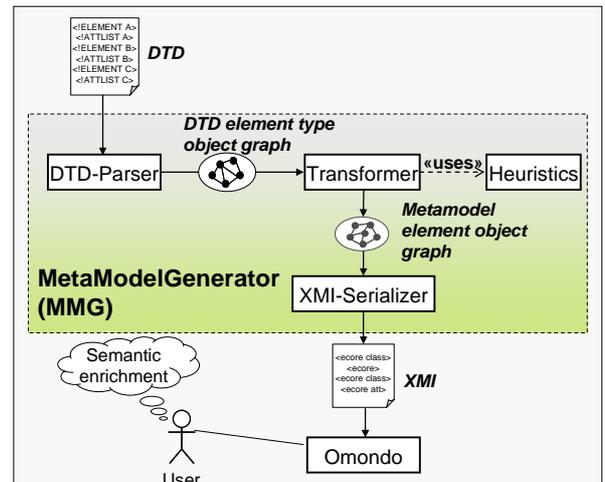
Figure 2: Architecture and Mode of Operation of the MMG
